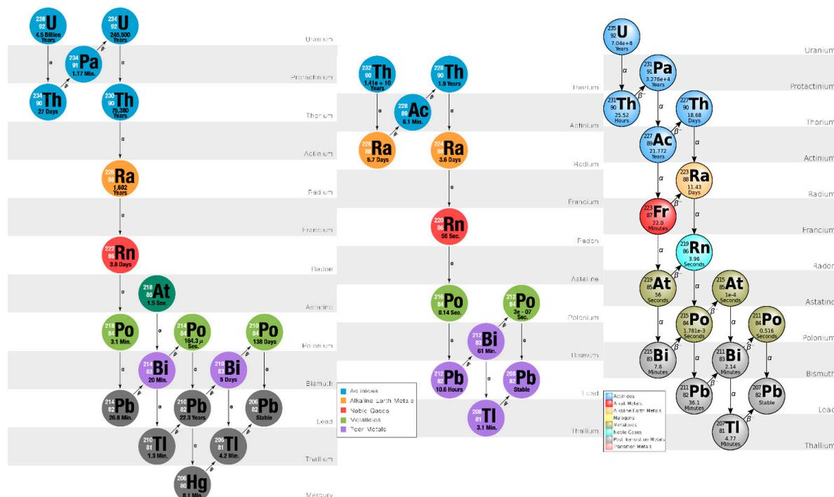
**Figure 1.** The decay trees of the main radon isotopes finished by stable elements. Left panel  $^{222}\text{Rn}$  chain (red circle); middle panel  $^{220}\text{Rn}$  named thoron (red circle); right panel  $^{219}\text{Rn}$  named actinon (turquoise circle). All images copyright © 2008–2024 the International Association of Certified Home Inspectors, Inc. (InterNACHI). <https://www.nachi.org/gallery/>.
