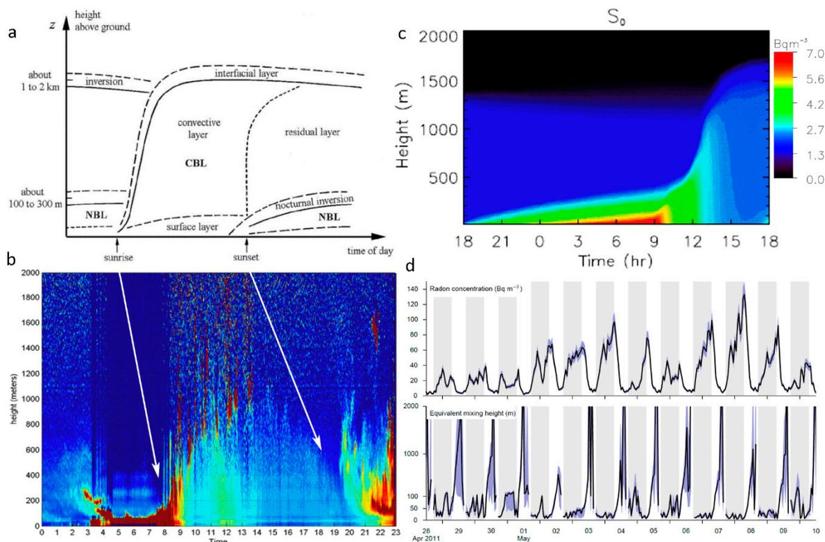
**Figure 3.** a – schematic presentation of the GBL daily dynamics [51]; b – lidar measurements of aerosol concentration in air [53]; c – modelling of the radon concentration  $S_0$  in local time as a function of GBL dynamics [54]; d – upper panel – radon in air concentration, bottom panel – equivalent mixing height during 12 days in April-May 2011 [55].
