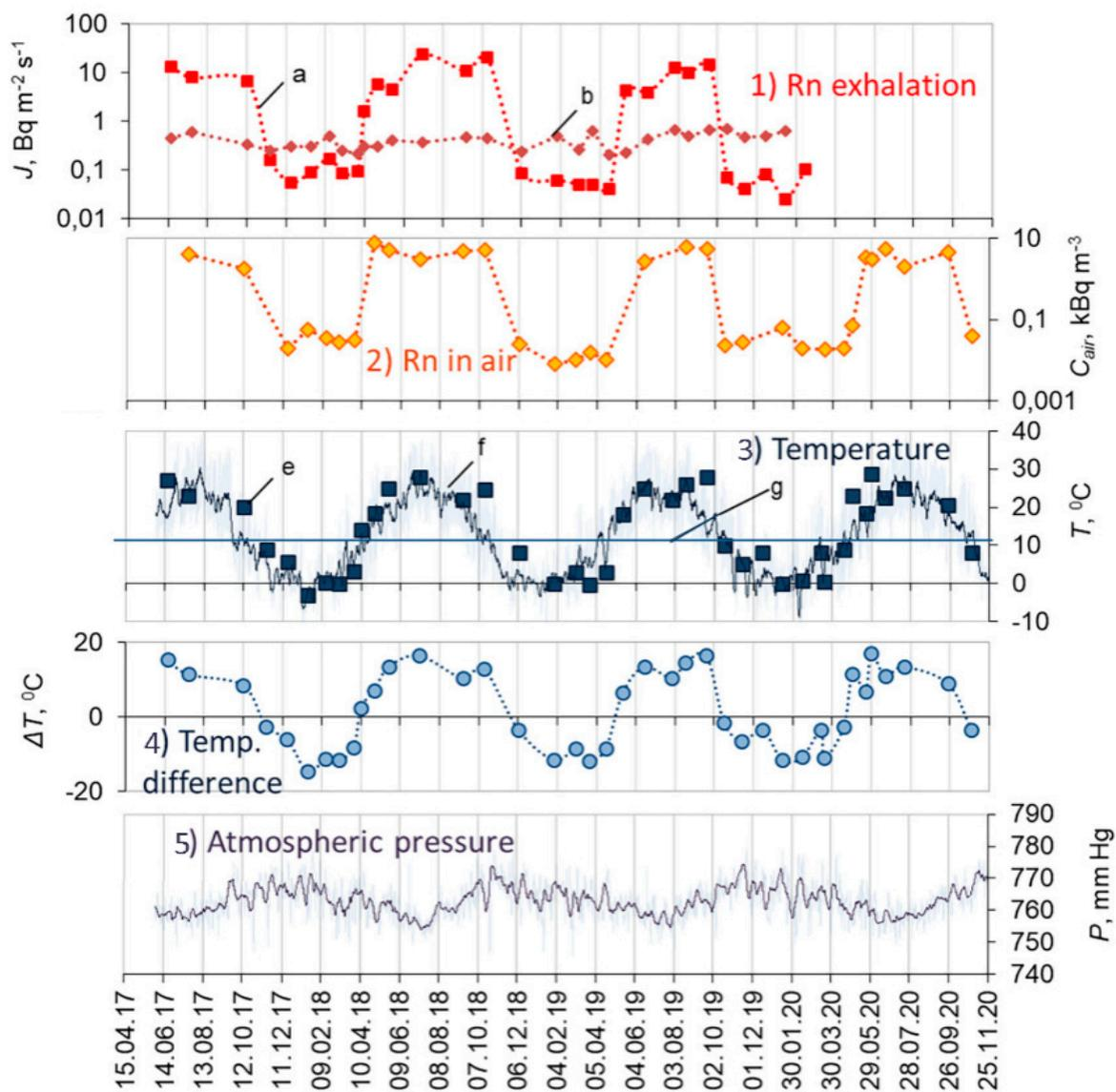
**Figure 5.** 1) – radon exhalation rate in the fault (a) and mean values outside the fault; 2) variation of radon in air over the fault; 3) air temperature (e – on monitoring site, monthly measurements ( $T_{\text{air}}$ ), f – data from Mineralnye Vody weather station (MVWS), g – average annual temperature inside the mine  $T_{\text{mine}} = 11.5^\circ\text{C}$ ) 4) temperature difference between the outside air temperature and temperature in mine; 5) atmospheric pressure.
