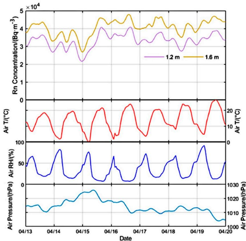
**Figure 2.** One-week measurement results of radon concentration (3 h moving average) in soil at 1.2 and 1.6 m, air temperature, air relative humidity and air pressure in typical spring days (April 13–20). The similarity of three publications results is due to the fact that the caves and wells have the direct contact with atmosphere [50].
